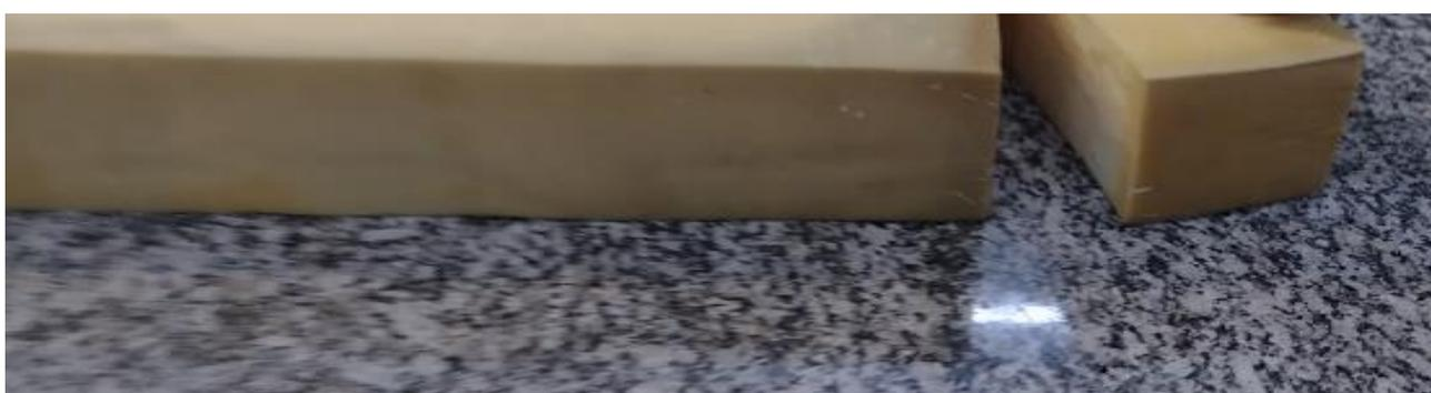
**FOTOS 4 A 6 – IRREGULARIDADES NA COLAGEM E PRESENÇA DE CASCA NA LÂMINA DO COLCHÃO**
